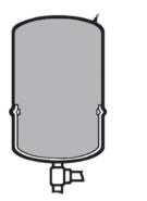
**Start-Up Cycle\*** Diaphragm is pressed against the bottom of the chamber.
